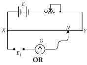
Following circuit was set up in a meter bridge experiment to determine the value X of an unknown resistance.
